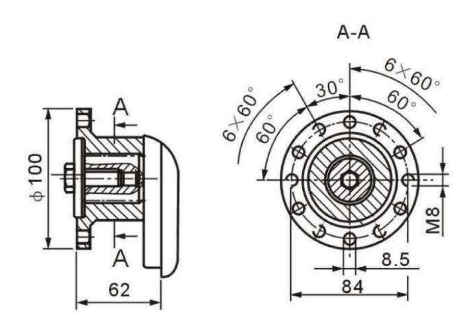
S Splined shaft 1 1/2in 23 T 16/32DP<sup>1)</sup> (SAE J744)
